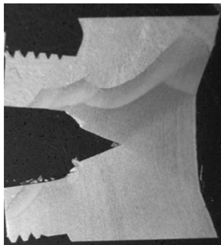
Figure 8-3 Crack-tip profile from a full-scale test specimen
