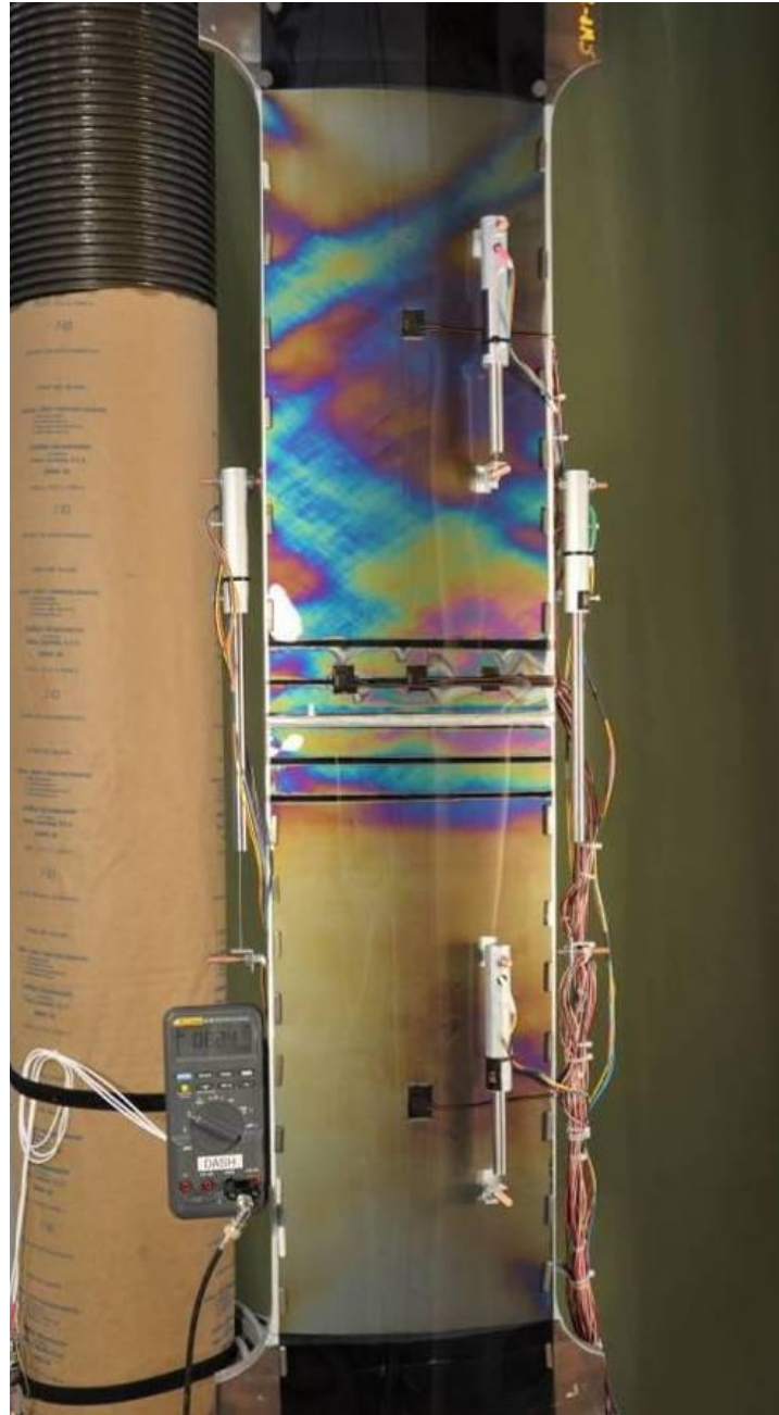
Figure 8.2 Photo-elastic image showing the non-uniform deformation on both sides of the girth weld [67]
